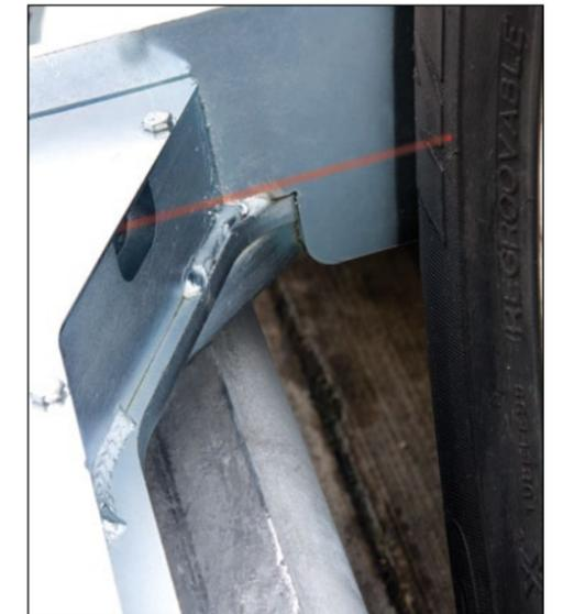
**Trailer Sensor:** IP67-rated photo cell sensor confirms presence of wheel in safe engagement range, and alerts both dock worker and restraint operator of premature disengagement.
