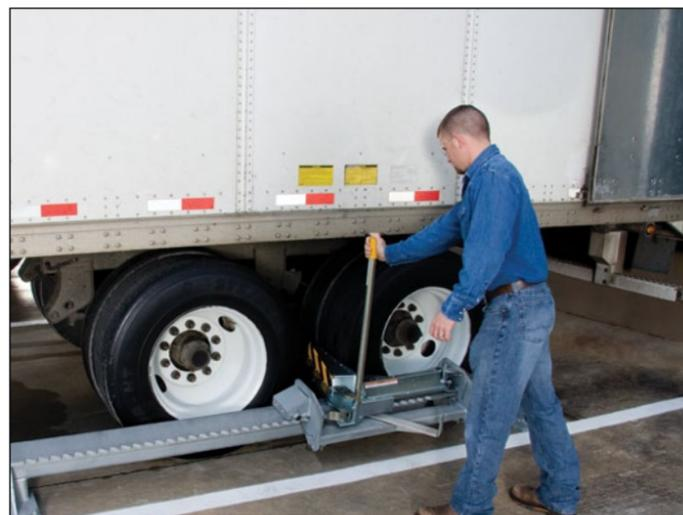
The operator slides the restraint carriage on the guide rail, positions it in front of the wheel, and pivots the restraining arm to lock it in place and secure the wheel.
