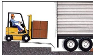
▲ **Trailer Walk:** During loading or unloading, the displacement of weight by the forklift can cause air-ride suspension trailers to move in an elliptical fashion, causing it to “walk” away from the dock in a more prominent motion.
