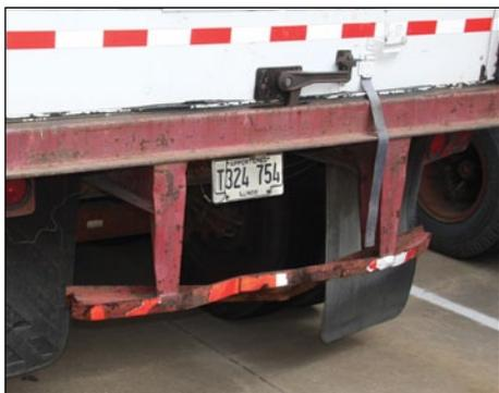
**Damaged Rear Impact Guards:** Some Rear Impact Guards have been bent or damaged over the years, rendering them impossible to restrain with a traditional vehicle restraint.
