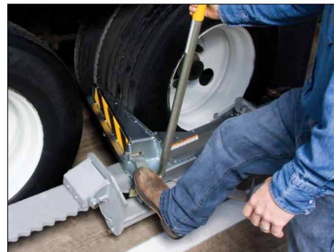
Once loading/unloading is complete, dock worker presses release button inside, alerting outside operator that it is safe to disengage wheel restraint. A simple press of the foot pedal disengages the restraining arm, rotating it back and away from the wheel.
