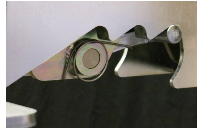
3-position slide lock limits trailer movement
